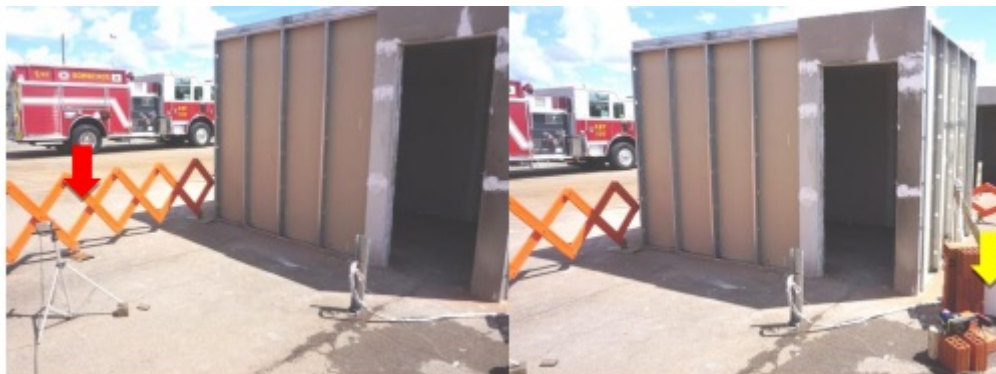
Figure 4 - Positioning of the high-definition (yellow arrow) and thermal (red arrow) cameras.
