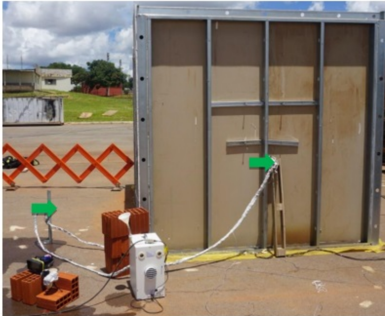
Figure 5 – Location of the heat flow sensors.
